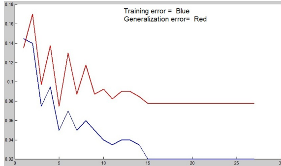
Figure 18: The training error (blue) and the generalisation error (red) against the size of the ensemble
